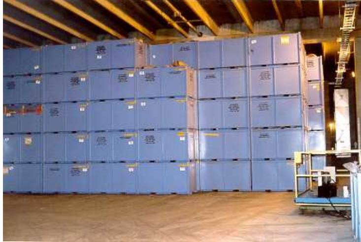
Figure 4: Steel boxes used to store LLW at the WWMF
